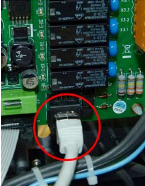
Pict. 1 - Serial bus connector RS 485 at the power supply
