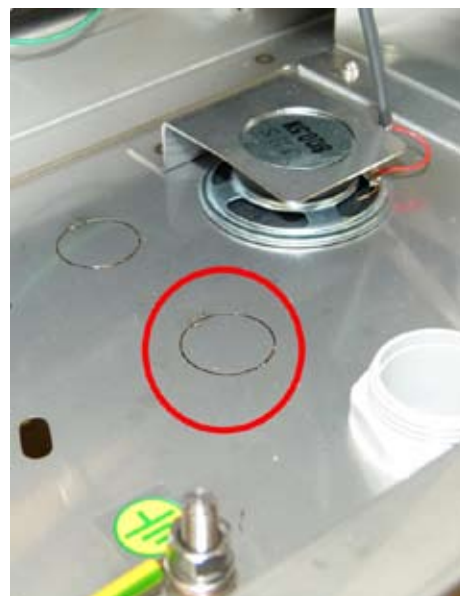
Pict. 4 - The opening for mounting of the UTP cable and its housing
